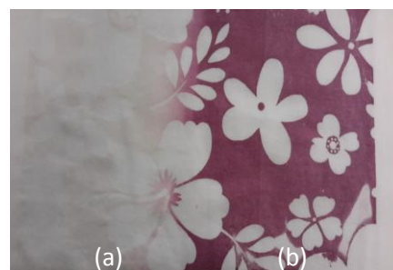
Figure 1: Photochromic textile coated with SNPs functionalized with a naphthopyran by screen-printing, (a) before and (b) after UV light exposure (1 min).
